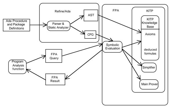
Figure 1. Basic FPA System Architecture
