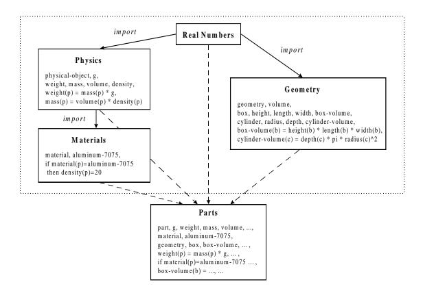
Figure 1: Construction of Parts Requirement Specification
