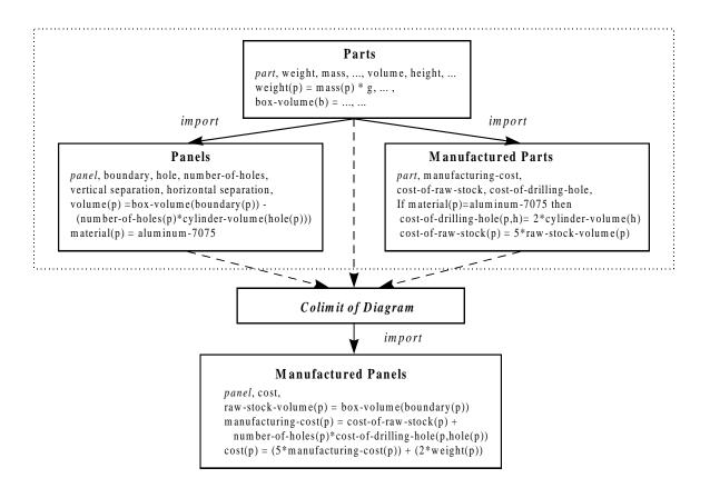
Figure 2: Construction of Manufactured-Panels Requirement Specification
