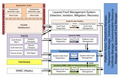
Figure 7. Layered fault management in F6MDA
