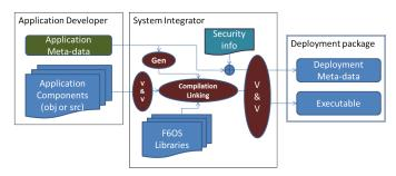
**Figure 11**. Application development and system integration for F6MDA
