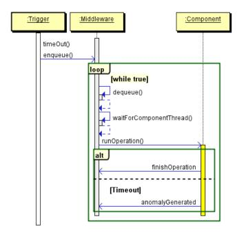
**Figure 6**. Interaction of a time trigger and component
